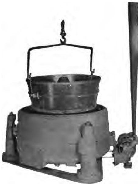
FIG. 37.—Centrifugal Machine. Showing basket about to be lowered into casing.
